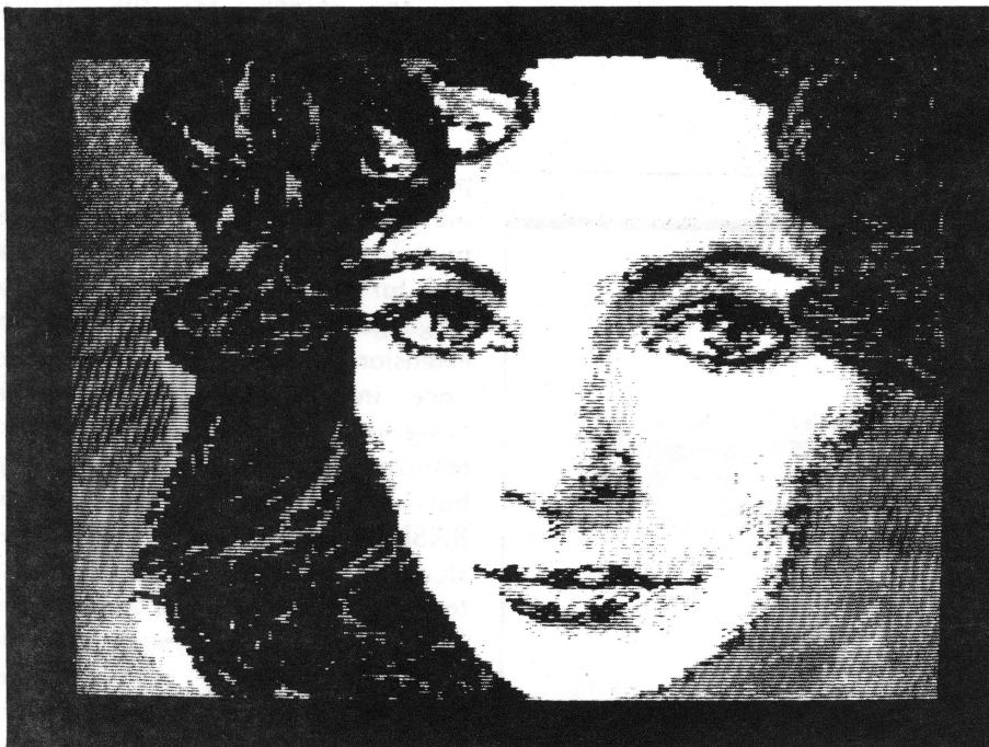
Photo 10: A talented artist with a digitizing tablet and the appropriate software can produce results like this by using blended colors in the Apple III's 140- by 192-pixel color mode.
