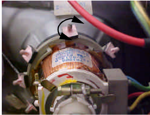
FIGURE 7. Geometry adjustment magnets (five visible; eight total)
